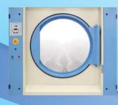
The large door opens 180 degrees making loading and unloading easy. The door glass is attached to the door without any gasket providing a long lasting door that offers security and low maintenance over the life of the machine. The door is provided with a safety switch that stops the machine when the door is open. A magnetic latch holds the door closed during operation. The door can be opened any time during operation for safety.
