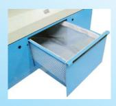
Large self-cleaning lint screens make maintenance easy. The screens are accessible from the front and located close to the exhaust fan, preventing fan clog up and eliminating fan vibrations. The lint filter is efficient and provides a good airflow that reduces the energy consumption. The microprocessor monitors the lint filter and stops the machine, should the lint screen become blocked.
